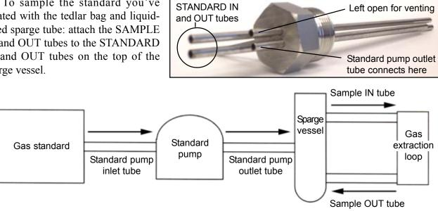
5. The extracted standard will return to the sparge tube to be regenerated for subsequent analysis.
