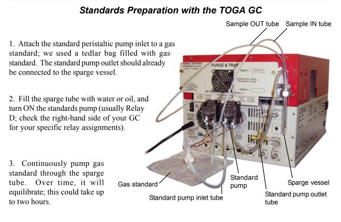
4. To sample the standard you've created with the tedlar bag and liquidfilled sparge tube: attach the SAMPLE IN and OUT tubes to the STANDARD IN and OUT tubes on the top of the sparge vessel.
