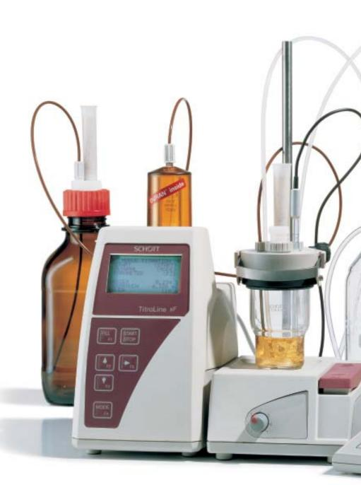
The TitroLine *KF* includes everything you need for water analysis according to Karl Fischer. The scope of supply includes the titrator, reagent bottle, titration stand TM KF, titration vessel, electrode and a starter kit (6 syringes with tubular needles, molecular sieve and three ampoules with a water standard specification). The waterproof mini keyboard TZ 2825 is available as an optional extra.
